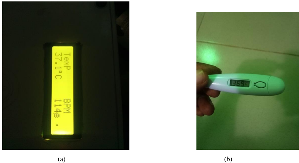
Figure 9: Heartbeat and temperature measurements of patient 2 (a) LCD displaying temperature and heart beats of patient 2 using the developed system (b) temperature reading obtained for patient 2 using axillary thermometer
