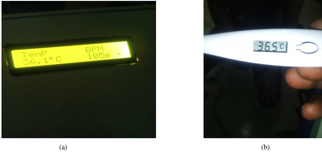
Figure 10: Heartbeat and temperature measurements of patient 3 (a) LCD displaying temperature and heart beats of patient 3 using the developed system (b) temperature reading obtained for patient 1 using axillary thermometer
