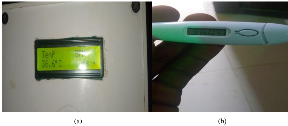
Figure 8: Heartbeat and temperature measurements of patient 1 (a) LCD displaying temperature and heart beats of patient 1 using the developed system (b) temperature reading obtained for patient 1 using axillary thermometer
