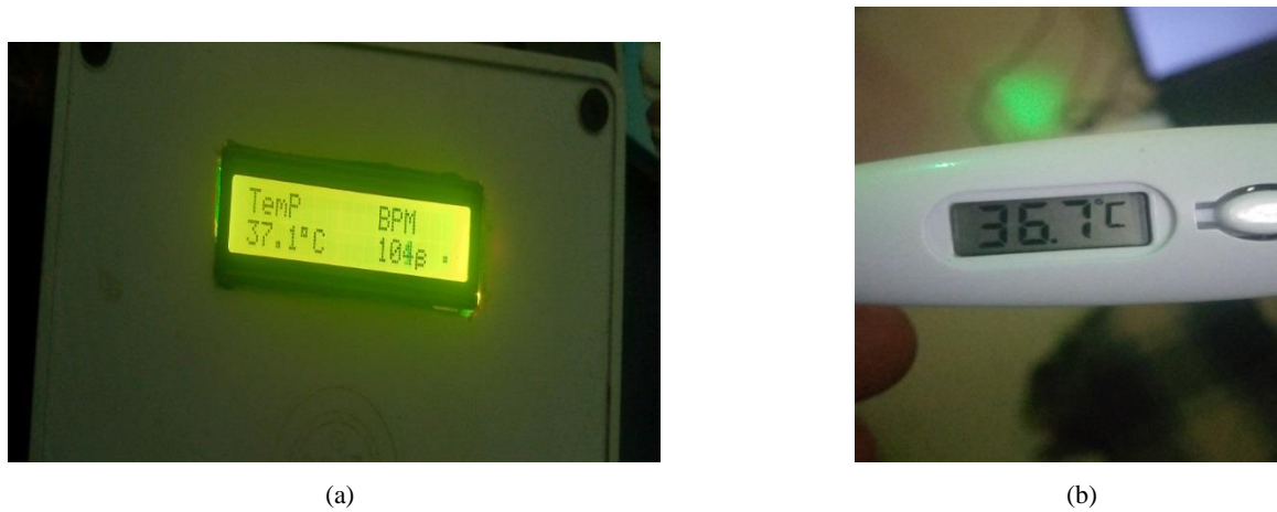
Figure 11: Heartbeat and temperature measurements of patient 4 (a) LCD displaying temperature and heart beats of patient 4 using the developed system (b) temperature reading obtained for patient 1 using axillary thermometer
